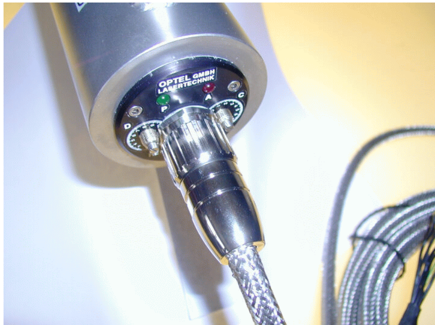
HLS Light Barrier Receiver with detachable Cable (optional)
